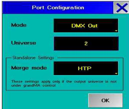
universe number - **and must be in a merge mode**. If DMX OUT is in merge mode "NONE" , the DMX signal will be inaccurate.
