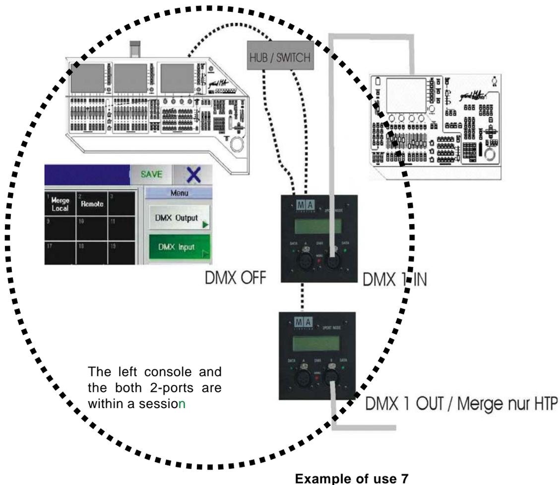
In this application example 7 – an output Universe is being controlled by the left console – the requirements for the stand-alone mode are not fulfilled, and only a restricted Merge mode is available. If on the left console, you set Universe 1 to LOCAL MERGE (in the menu TOOLS / DMX CONFIGURATION / DMX INPUT) you will only have the HTP option for the Merge mode.
