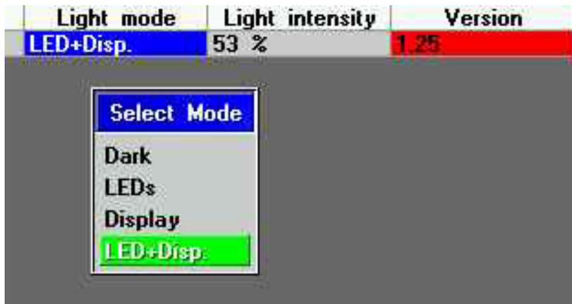
**DARK** Will switch off LEDs and display lights (independently from the **Light Intensity** setting).
